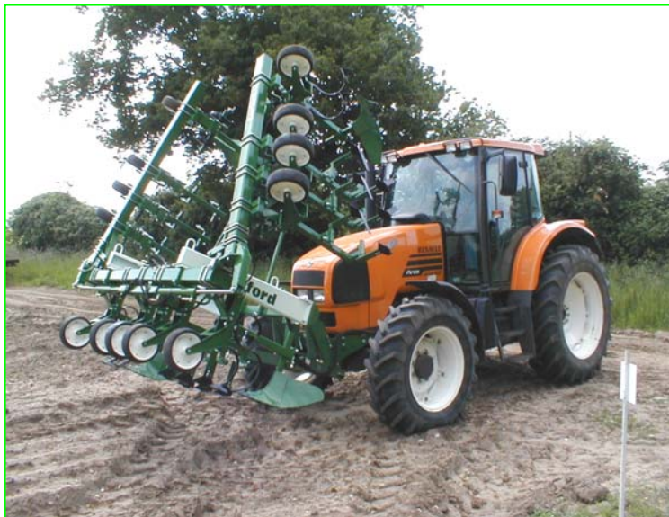
6 metre hydraulic folding frame
