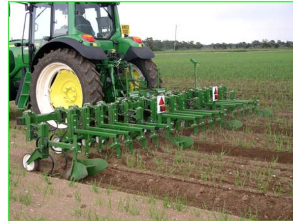
Robocrop hoeing triple beds of onions
