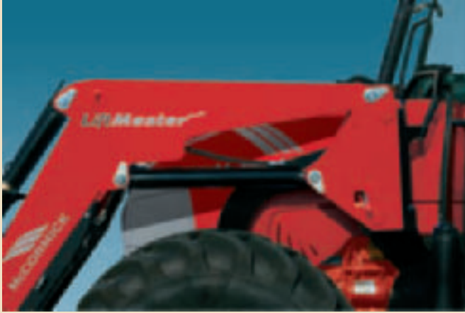
The No Levelling ECO (10 – 15 - 20 – 30 – 40 series) and No Levelling TOP (10 – 15 - 20 – 30 – 40) versions come without self-levelling system for 45 to 150 HP tractors.
