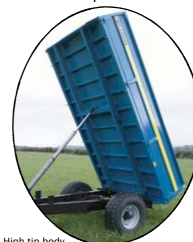
High tip body with close spaced floor supports
