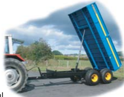
Close coupled reinforcing floor supports for added floor strength
