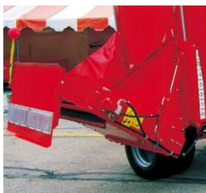
Discharge chain conveyor or belt conveyor with magnet.
